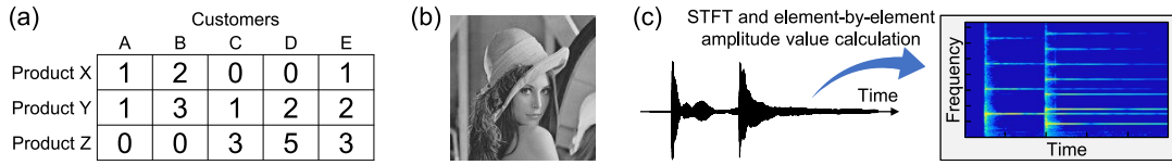
Fig. 1.1 Nonnegative matrices appearing in real situations: (a) customer purchase data, (b) monochrome image data, and (c) time-frequency amplitude of audio signals.
