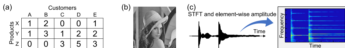
Fig. 1.2. Nonnegative matrices appearing in real situations: (a) customer purchase data, (b) monochrome image data, (c) time-frequency amplitude of audio signal.
