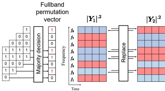
Fig. 8. Solving permutation problem by replacing frequency-wise components on the basis of the fullband permutation vector.
