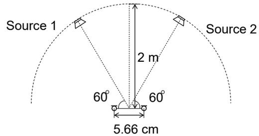
Fig. 9. Recording condition of JR2 impulse response.
