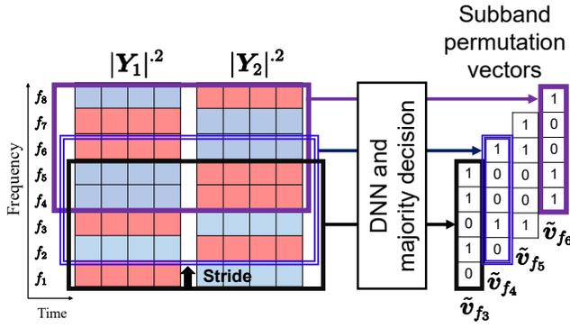
Fig. 6. Estimation of subband permutation vectors in all frequency bins. Subband is shifted with stride length and several overlaps. Similarly to time-frame axis, majority decision is performed for each frequency bin.
