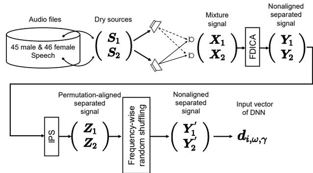
Fig. 10. Process flow of producing input vectors for DNN.
