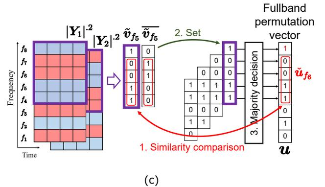
Fig. 7. Reconstruction of fullband permutation label: (a) initialization step, (b) second step, and (c) last step, where similarity comparison is based on MSE. This process is performed to associate DNN predictions (zeros and ones) with each source component.
