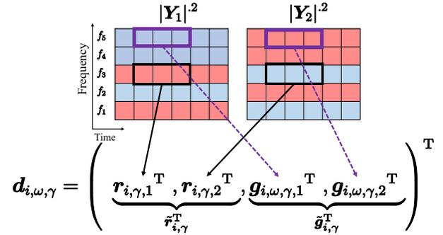
Fig. 2. Input vector of DNN. Matrices  $|\mathbf{Y}_1|^2$  and  $|\mathbf{Y}_2|^2$  are separated power spectrograms with permutation problem, and red and blue binwise activations (rows of  $|\mathbf{Y}_1|^2$  and  $|\mathbf{Y}_2|^2$ ) depict sourcewise components, e.g., red and blue slots respectively correspond to first and second source components.
